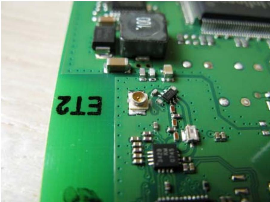
Now, carefully remove the thin coax connector from the printboard. Now, the old fixed antenna is free and can be removed.
