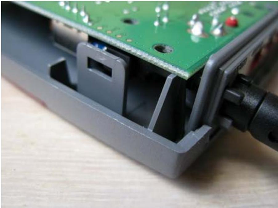
Let's start with the actual modification. It is very easy to open the Fritz!Box. There are four clips, no screws. With a small screwdriver just push the clips sideways. Be careful. If you perform the right movement, the enclosure opens very smoothly. Also, closing it again is just as simple.
