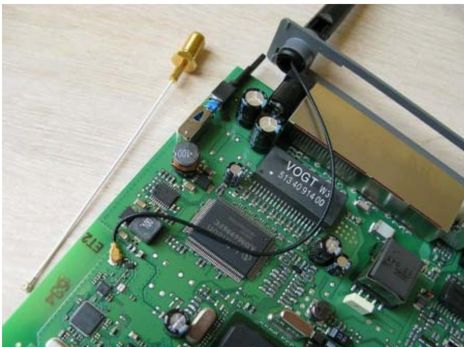
After you open the case, this is what you see. The backplate easily comes loose after you open the enclosure. The antenna sits in a plastic tube in the rear side. The new chassis-connector and cable combo lies beside the case.
