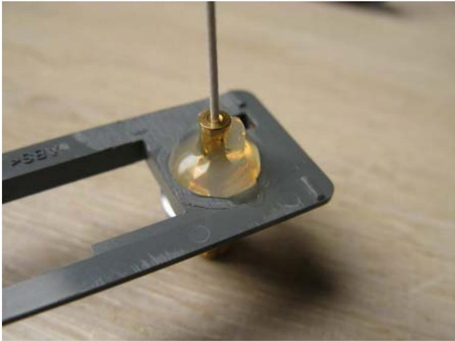
After cooling down, you can click the new printconnector in place on the prinboard.
