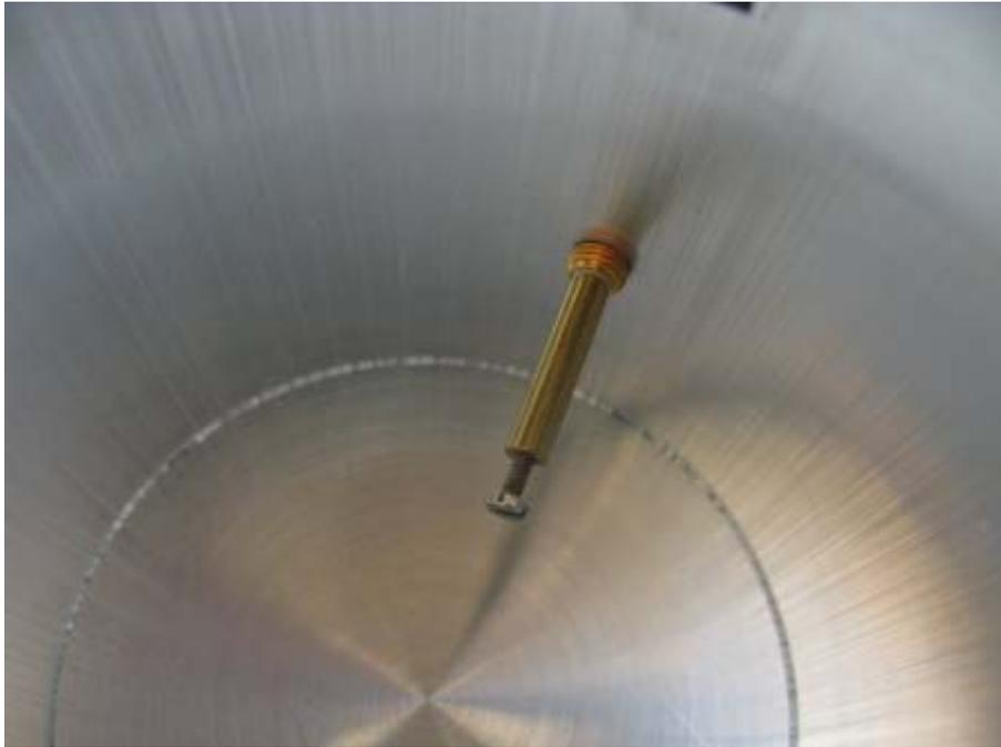
Take a look into the antenna cavity. The metal pin is the actual antenna. With the screw the antenna is tuned to the right frequency. Johannes provides measuring reports for each individual antenna. The can around the antenna put the signals in the right direction and adds to the antenna gain. With the screwholes in the backside you can choose either for horizontal or vertical polarisation.
