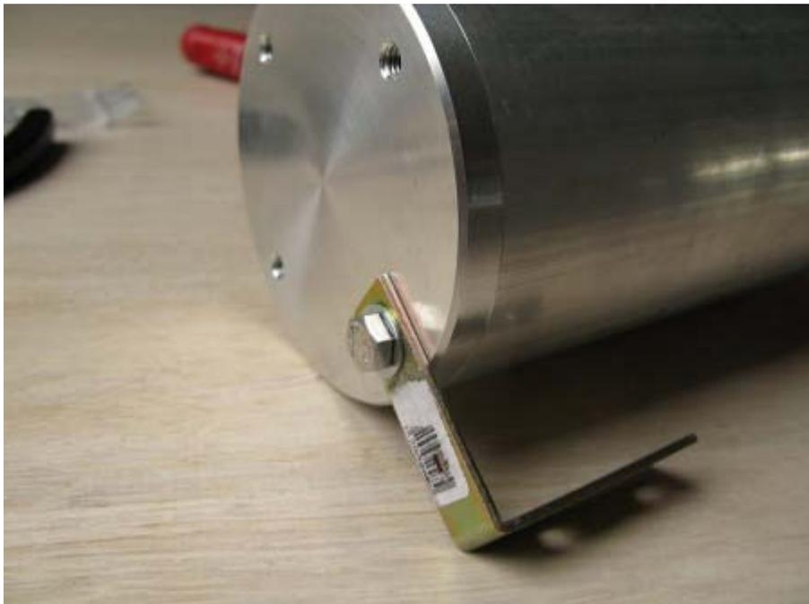
As you can see, there are four mounting holes on the backside of the antenna. This gives you the possibility to radiate your W-LAN signals either horizontally or vertically. If you use only one screw in the bracket, you can play with antenna pointing direction for the best results!
