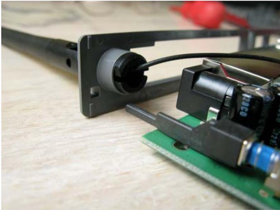
Now, remove the antenna from the rear panel. Again, that is very simple. Just squeeze the halves in the antenna foot a bit, and slide it out. Done! The Fritz!Box is a very clever and service friendly designed machine.
