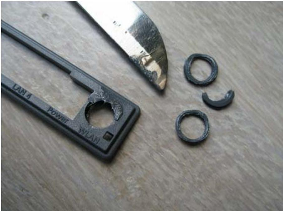
With a small sharp knife and a file you can smooth up the backpanel. Be very careful if you use a heated knife. I had to glue the new SMA connector in. The backplate was too thick to fix the new connector, and leave enough thread sticking out for a secure connection. Even with thin metal rings, the combination with washers and locknut was too thick.
