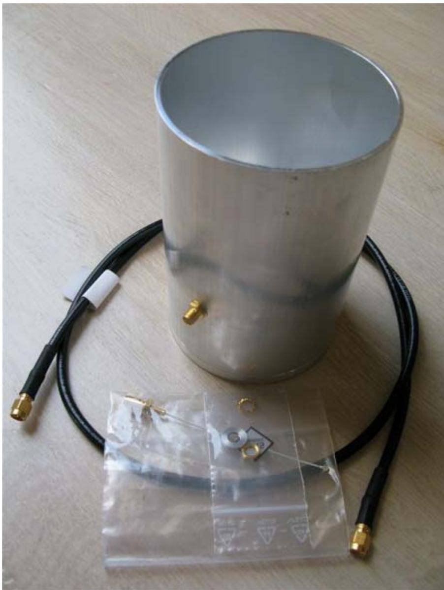
These are the new parts: antenna, coax cable, and modification kit
